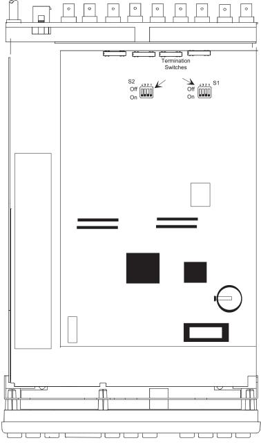
Most components removed for clarity.TC8278 Series is shown. TC8277 Series has only one termination DIP switch.
